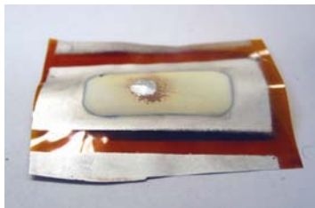
Figure 20. A flexible UT using polyimide film as the substrate.
