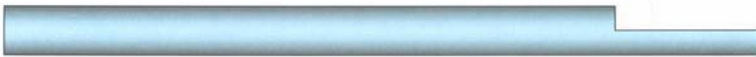
Figure 2 (b). Torsional T sensor design from a 2001 undergraduate student project at Tufts University. Students [9] started with a 4.76-mm ( 3/16'' ) diameter cold rolled steel rod, milled one end to create a semicircular cross section of length 25.4 mm, and measured the torsional transit time between the shoulder echo and the end echo. (A larger-diameter notched bar was used in 1947 for bulk guided wave determinations of elastic properties [19].) In [9], torsional calibration was conducted from room temperature to 650^\circ\text{C} . The sensor was first placed in a SS (stainless steel) sheath. The sheath was heated with a propane torch. The reference T was a thermocouple in contact with the sensor. Among results obtained in [9]: (1) K_{SH} \approx 0.77 ; (2) From \sim 140 to 440^\circ\text{C} , torsional transit time increased linearly as T increased, \sim 5 ns/ ^\circ\text{C} for one round trip in the sensor.
