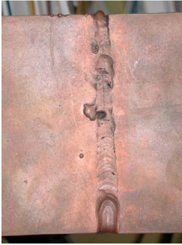
Figure 4a. A photo of a copper welding sample which shows an open crack just to the right and above a lump of copper on the surface.
