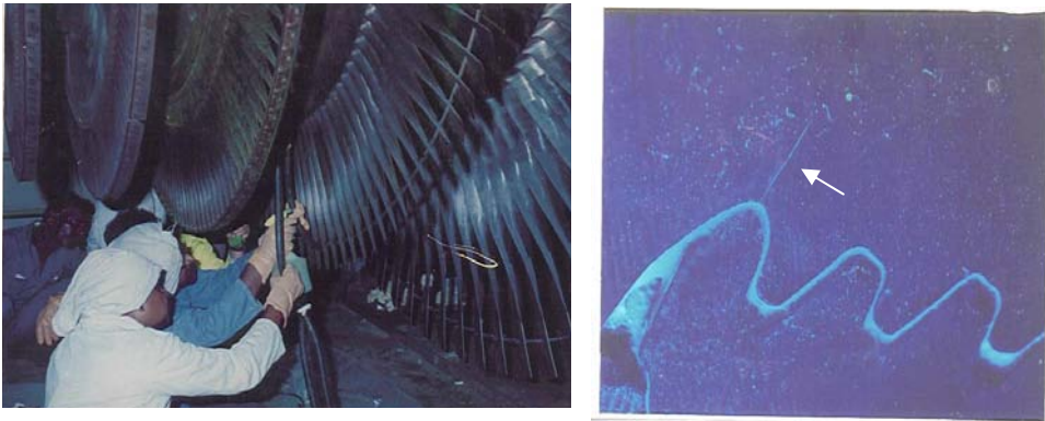
Figure 5. Fluorescent MP testing of a steam turbine rotor and typical indication from a tight fatigue crack in the 'fir-tree' root region of a low-pressure blade.
