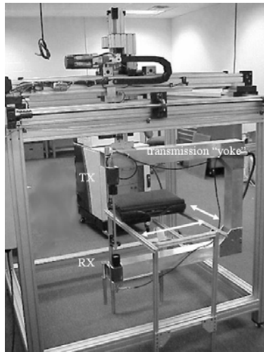
Figure 3. QA1000 scanner configured in transmission configuration with overhead X-Y raster scanner and "yoke" mounted transmitter (TX) and receiver (RX).
