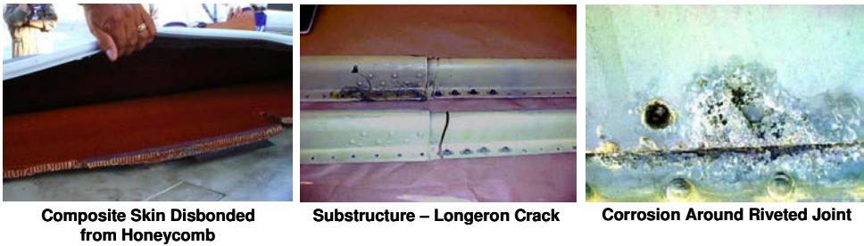
Figure 1. Sample Disbond, Crack and Corrosion Damage in Aircraft Structure.
